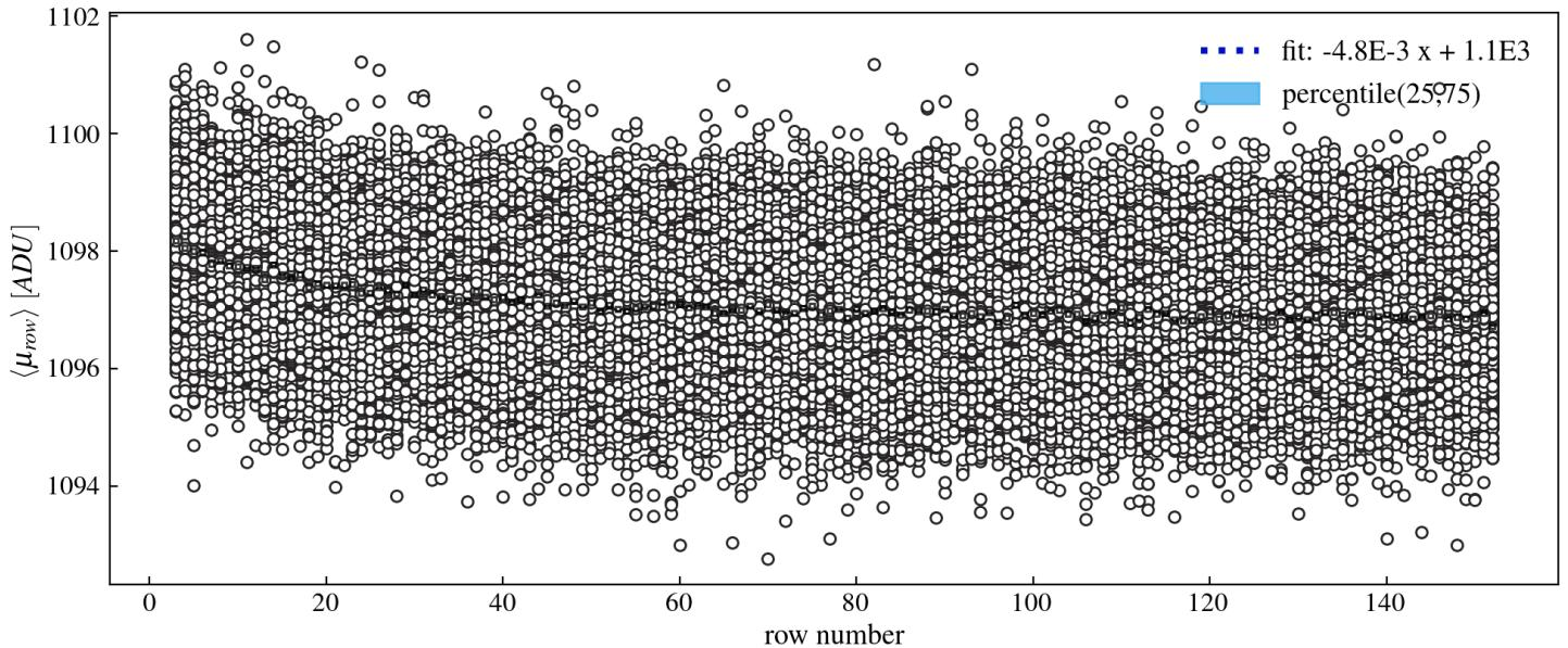
Figure 12: PedestalSubtractionProcess: mean pedestal vs file (gauss fit)
