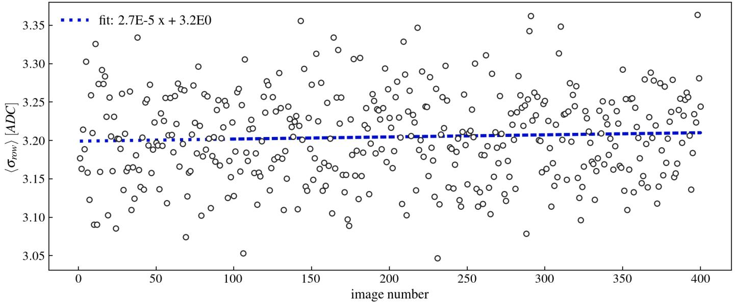
Figure 11: PedestalSubtractionProcess: mean sigma vs file (gauss fit)
