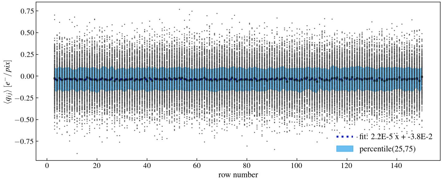
Figure 1: Active Area. Median dark current (only  $q_{i,j} < q_i^{th}$ ) vs row
